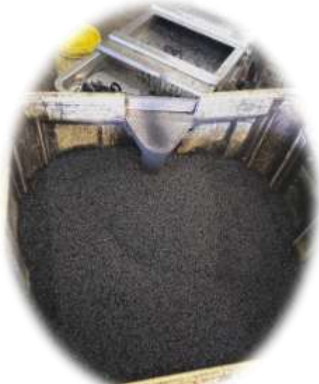
5. Pelletising extruded HDPE plastic
