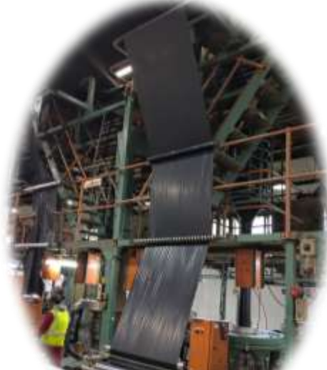
6. Manufacturing plastic refuse bags from recycled HDPE
